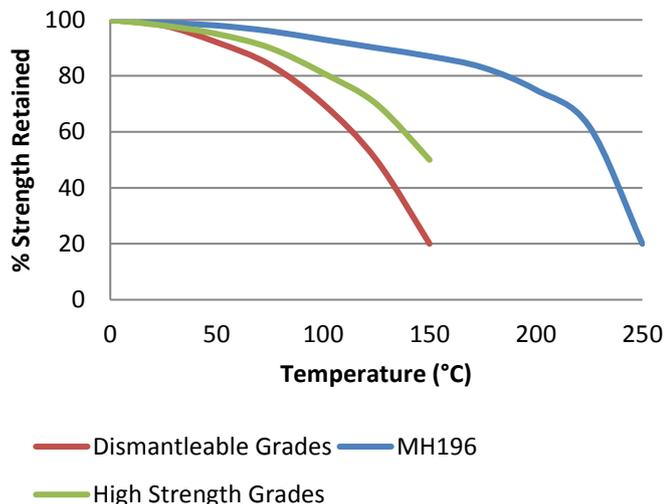
*"Hot strength" Breakaway strength on M10 Zinc plated bolts according to ISO 10964. Cured at 23°C for 24 hours then conditioned for 30 minutes at testing temperature.*
