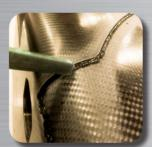
used for high strength bonding of carbon fibre body panels
